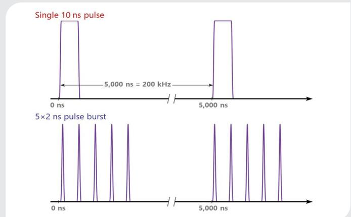
Figure 1. In burst mode, the laser emits a short series of pulses (burst sub-pulses) rather than an individual pulse. Each pulse burst can have nearly the same total energy as a single (longer) pulse at that same repetition rate.
