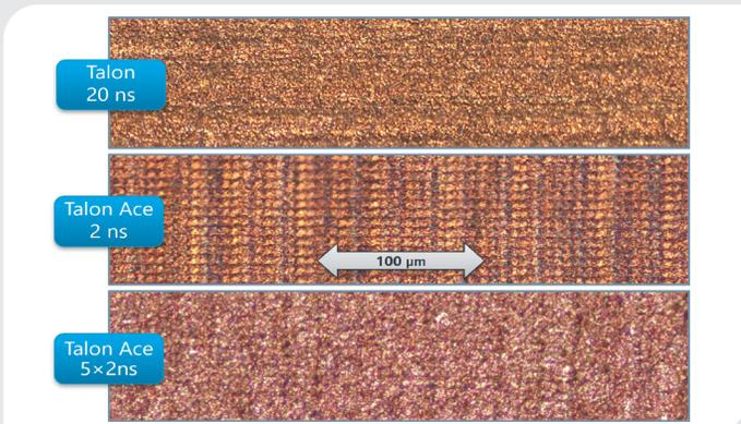
Figure 3. Closeup optical microscope photos showing machined surface quality for 2- and 20-ns single pulse outputs as well as a 5x2ns burst output.
