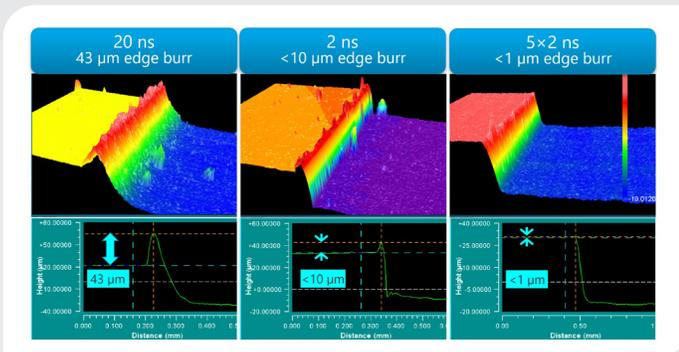
Figure 4. Optical surface profilometry reveals decreasing edge burr when going from 20 to 2 ns pulse widths, and further reduction with a 5x2 ns burst output.
