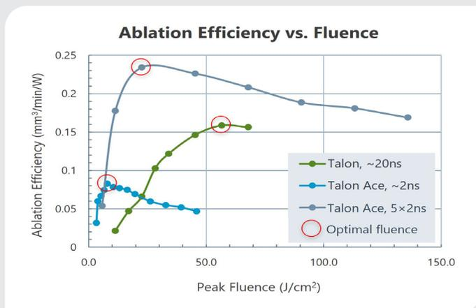
Figure 2. Ablation efficiency data illustrates the importance of pulse width and the benefit of using pulse bursts when processing copper.
