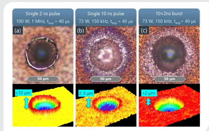
Figure 5. : For equal or lower average power, a 10x2 ns burst offers superior results for flex PCB top copper via opening compared to single 10 ns and 2 ns pulses.
